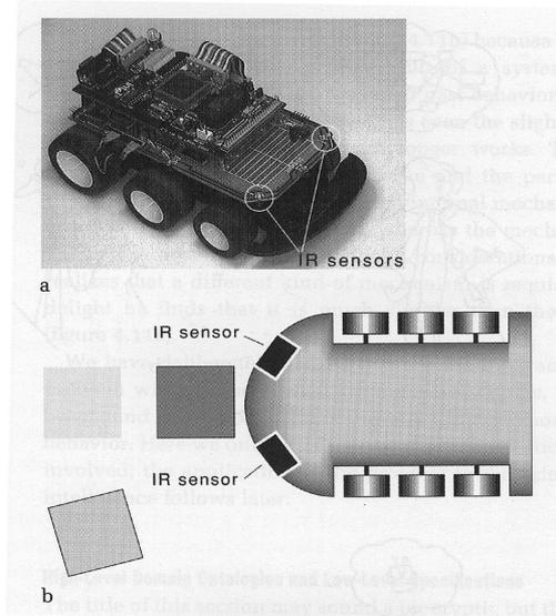
Figure 2 (a) Picture of a Didabot. (b) Infrared- Sensor configuration of Didabot.
