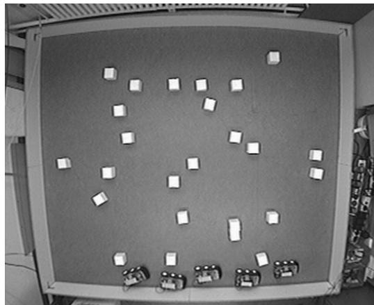
*Figure 1: Didabots in their arena. There is an arena with a number of Didabots, typically 3 to 5. All they can do is avoid obstacles.*
