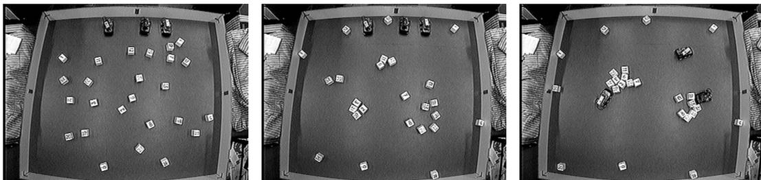
Figure 3: Example of heap building by Didabots. Initially the cubes are randomly distributed. Over time, a number of clusters are forming. At the end, there are only two clusters and a number of cubes along the walls of the arena.
